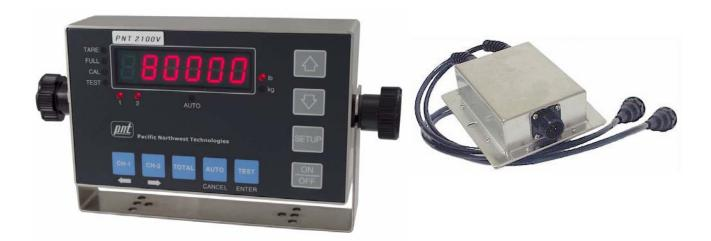
The **Model 2100V** In-cab Meter from PN Technologies is used in all on-board scale applications requiring dual channel weight displays. Total vehicle weight is displayed as well as individual tractor and trailer weights. The PNT 2100V meter can be set to cycle automatically between individual channel weights and total weight displays. The operator can press the cycle button at any time to stop and monitor any channel desired.
